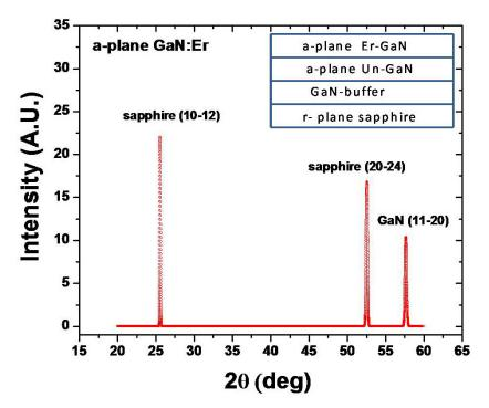
Fig. 1. X-ray diffraction  $\theta$ -2 $\theta$  scan of *a*-plane Er doped GaN epilayer grown on *r*-plane sapphire substrate. Inset: Schematic layer structure of a-plane Er doped GaN epilayer (GaN:Er).
