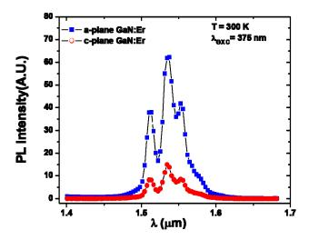
Fig. 2. Comparison of room temperature (300 K) Er-related PL spectra near1.54 μm between *a*-plane and c-plane Er doped GaN epilayers. The excitation wavelength used was 375 nm.
