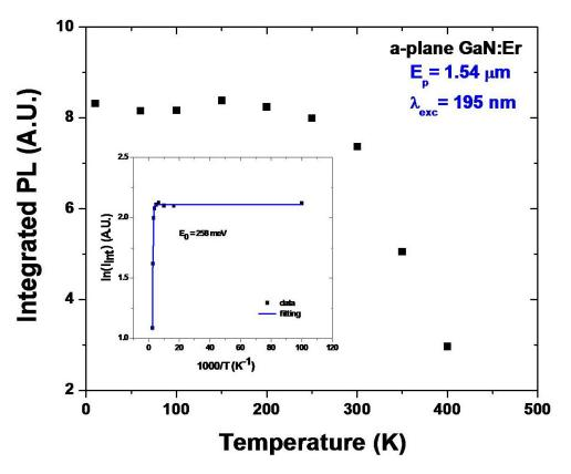
Fig. 5. Integrated PL emission intensity of the 1.54  $\mu$ m emission of *a*-plane Er doped GaN vs sample temperature. Inset: Arrhenius plot of the integrated PL intensity of the 1.54  $\mu$ m emission. The solid line in the plot is the least squares fit of the measured data to Eq. (1). The excitation wavelength used was 195 nm.
