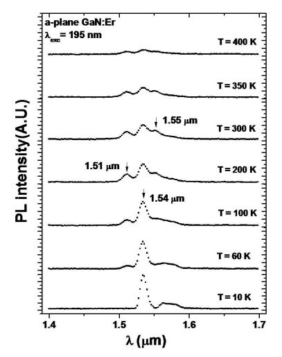
Fig. 4. PL spectra of the 1.54  $\mu$ m emission of *a*-plane Er doped GaN measured at different temperatures from 10 to 400 K. The excitation wavelength used was 195 nm.
