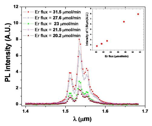
Fig. 3. Room temperature PL spectra of *a*-plane Er doped GaN epilayers showing the variation in the emission intensity of the Er related emission at 1.54  $\mu$ m with the Er molar flux employed during the growth. The excitation wavelength used was 375 nm. Inset: The PL intensity at 1.54  $\mu$ m as a function of Er molar flux.
